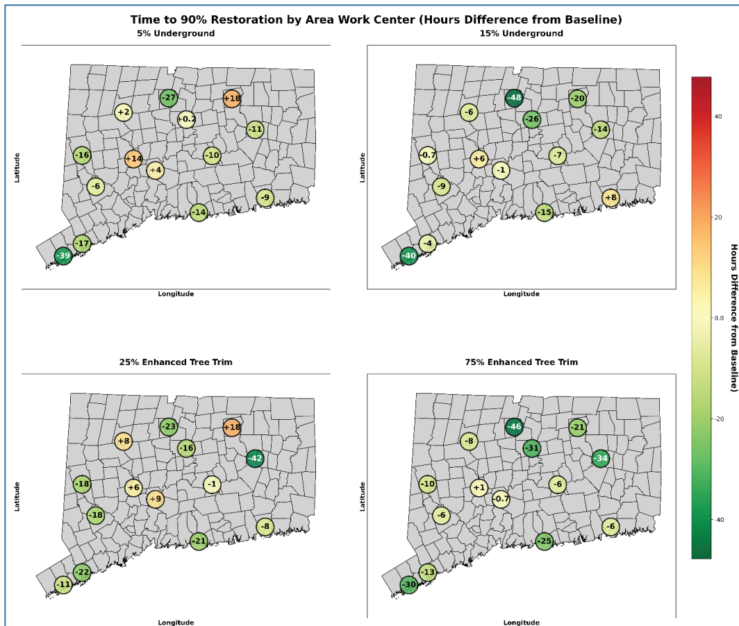
Figure 16. Change of restoration time by Area Work Center (AWC): the numbers represent the differences (in hours) for achieving 90% of customer outage restoration, with respect to the baseline scenario. Green circles indicate faster restoration, while orange/yellow circles show areas with minimal improvement or even slight delays.
